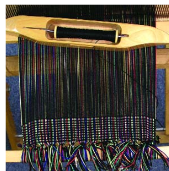
h. Edge threads are too tight
