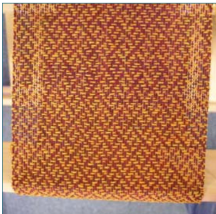
c. Weave at an open sett of 10 ppi.
