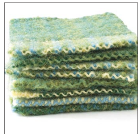
f. A fine weft and heavy warp can produce weft take-up of more than five percent.
