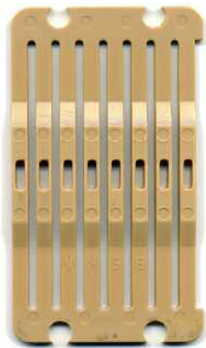
c. Section of a rigid heddle
